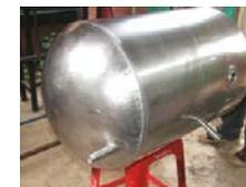
Pressurized tank from SUS304 stainless steel.
