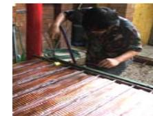
Welded and assembly under strict quality control. Every panel fulfills a 6 bar pressure test.
